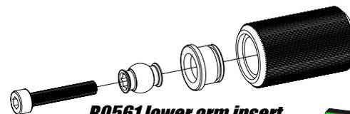
**B0561 lower arm insert tool (assemble/disassemble) Opt**
