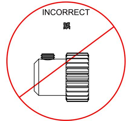
Please be sure the set screw of the pinion doesn't stand out of the pinion. This will lengthen the durability of the front belt.
